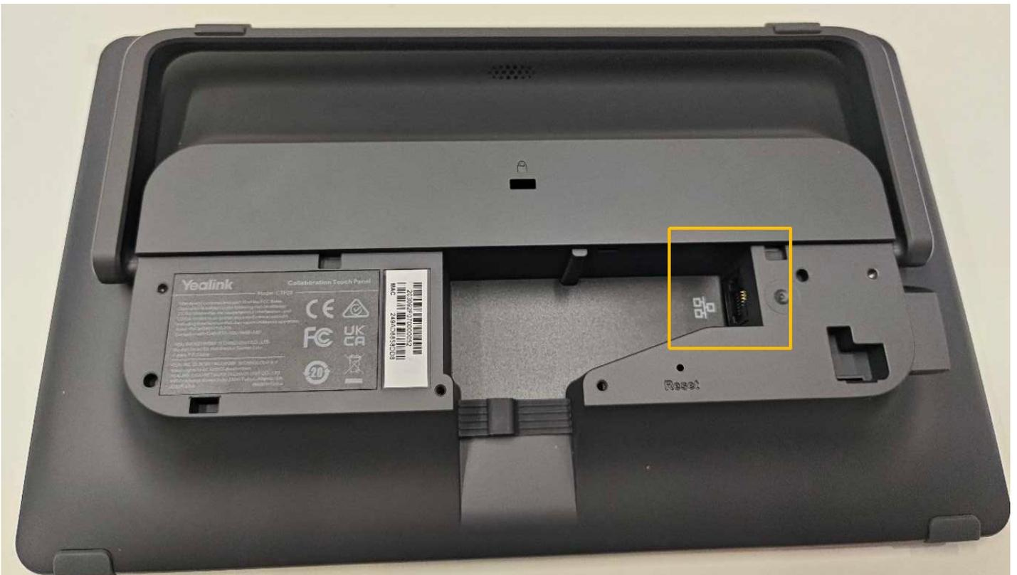
b) Use a network cable to connect the **Ethernet IN** interface of the **PoE power supply** to the LAN.
