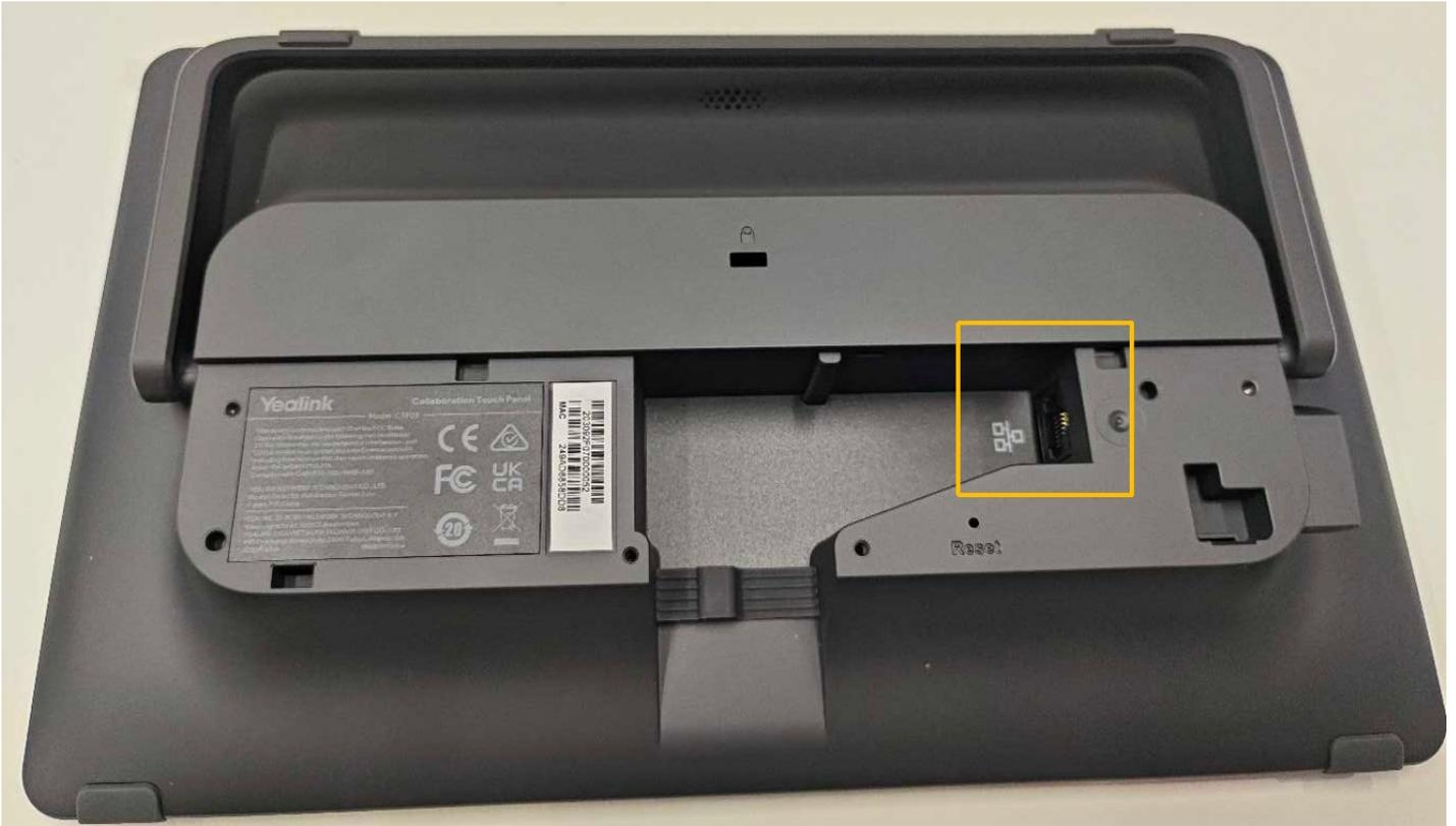
b) Use a network cable to connect the **Ext Touch port** of the MTouch Plus to the same LAN as the MTouch Plus-EXT.
